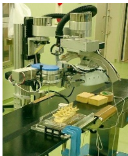
Fig. 2. Developed Needle Insertion Robot
