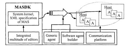
Figure 1. MASDK software tool components and their interaction
