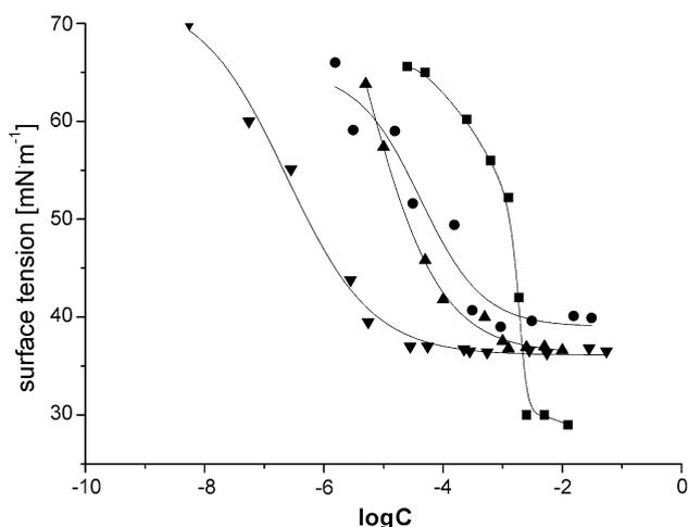
**Fig. 2** Surface tension isotherms for ■ P10S3, ● P12S3, ▲ P14S3, ▼ P16S3
