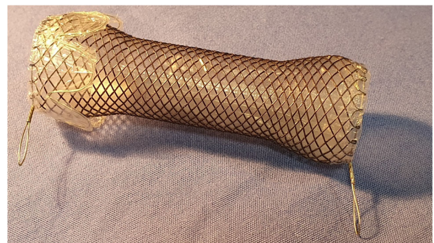
Figure 10 Ella-HV oesophageal stent demonstrating forward facing wings paired with flared ends to reduce the risk of stent migration. The stent body diameter is 18–20 mm with a flare outer diameter of 25 mm and length 85–150 mm [114].
