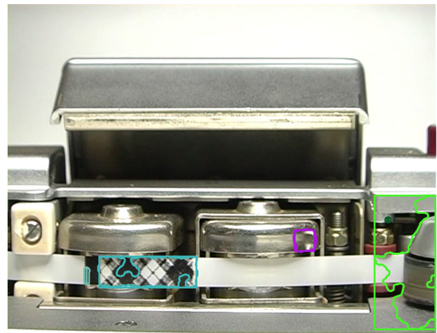
Fig. 10 An intermediate step in the detection of “anomalies” on the tape. Three anomalies have been detected, as shown by the colored contours ; false positives will be discarded in a next step of the algorithm (color figure online)
