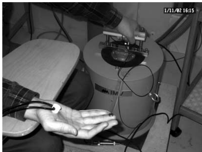
Fig. 1. Experimental set-up. While sitting upright in a chair, the subject's left hand was subjected to a 125-Hz sinusoidal vibration of 50 \text{ m/s}^2 (rms) for 3 min. Measurements were made of palmar sweating and skin temperature of the palm and fourth fingertip, respectively, of the subject's right hand
