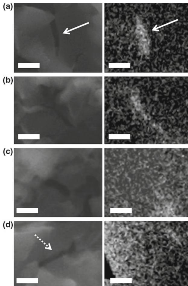
**Fig. 4** Comparison between small sections of SEM images (*left column*) and EUV images (*right column*) showing different areas of the sample. **a, b** Some cracks, as small as 100 nm, in the sample are deep all the way to the membrane and can be seen in both SEM and EUV images (marked with *white arrows* and **c, d** some of the features (marked with *dotted arrow*) are visible in the SEM images but are not present in the corresponding EUV image. *Scale bar* is 2  $\mu\text{m}$
