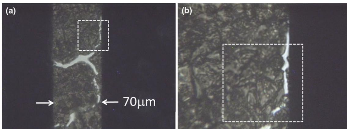
**Fig. 2** Optical images of thin Si membrane with NaCl crystals deposited on top with **a** 40 $\times$  (NA = 0.65), **b** 100 $\times$  (NA  $\sim 1$ ) objectives. Dashed boxes indicate the size of object region imaged with the EUV microscope
