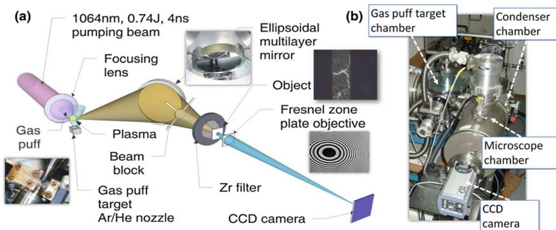
**Fig. 1** a Scheme (not to scale) and b photograph of the EUV microscope using a laser-plasma EUV source based on gas-puff target
