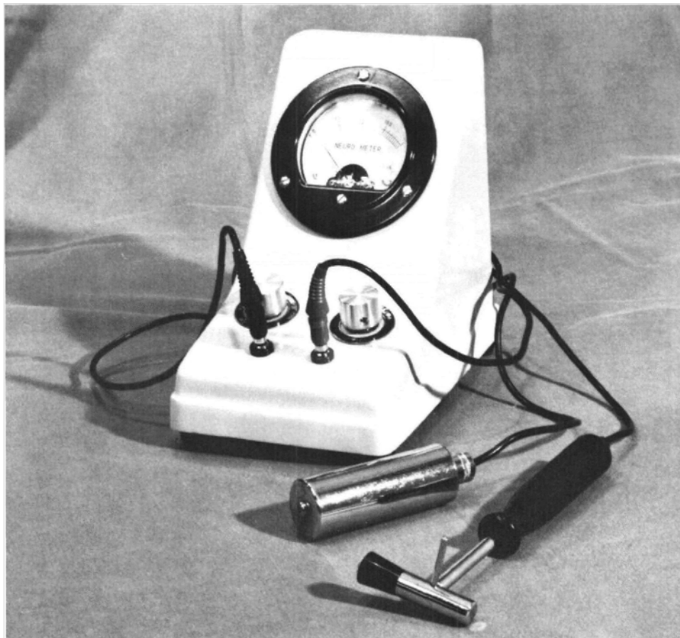
FIGURE 2. Neurometer LC type. This equipment is used to stimulate with weak direct current through the inserted needle, also it can be used to find the points of low electrical skin resistance.
