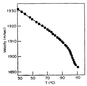
Figure 1. Longitudinal wave velocity in amorphous  $Ge_{15}Se_{85}$  sample plotted against temperature.
