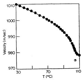
Figure 2. Transverse wave velocity in amorphous  $Ge_{15}Se_{85}$  sample plotted against temperature.
