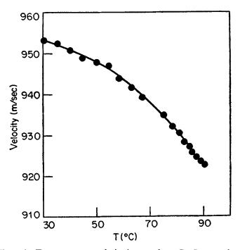
Figure 4. Transverse wave velocity in amorphous  $Ge_{10}Se_{90}$  sample plotted against temperature.
