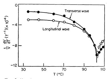
Figure 5. Normalized temperature coefficient of longitudinal and transverse wave velocities in amorphous  $Ge_{15}Se_{55}$  sample plotted against temperature.
