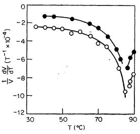
Figure 6. Normalized temperature coefficient of longitudinal and transverse wave velocities in amorphous  $Ge_{10}Se_{90}$  sample plotted against temperature.
