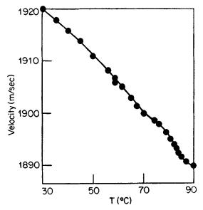
Figure 3. Longitudinal wave velocity in amorphous  $Ge_{10}Se_{90}$  sample plotted against temperature.
