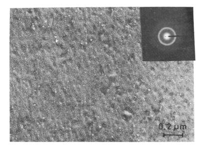
Figure 1. Electron micrograph of nominal composition  $Y_2GdFe_5O_{12}$  heat-treated at 700°C for 1 hr. Inset shows the corresponding electron diffraction.
