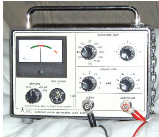
Fig. 13.31 This temporary pacing box from APC cardiovascular has a key to enable X3 pacing for overdrive pacing
