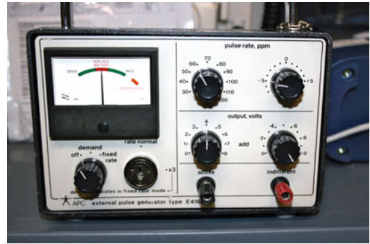
Fig. 13.27 Temporary pacing box from APC Medical
