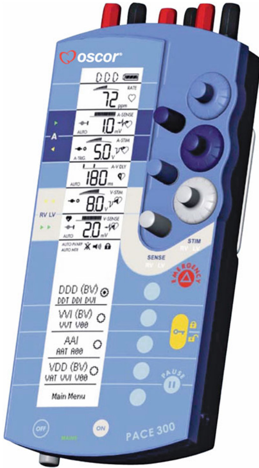
Fig. 13.30 PACE 300 three-chamber temporary pacemaker (Osypka) has a large range of features including AUTO SENSE for automatically tracking P/R wave peak amplitudes and adjusting atrial and ventricular sensitivities. An optional function automatically adjusts the settings for AV delay, PVARP and MTR depending on selected stimulation rate. A wide range of pacing modes are available
