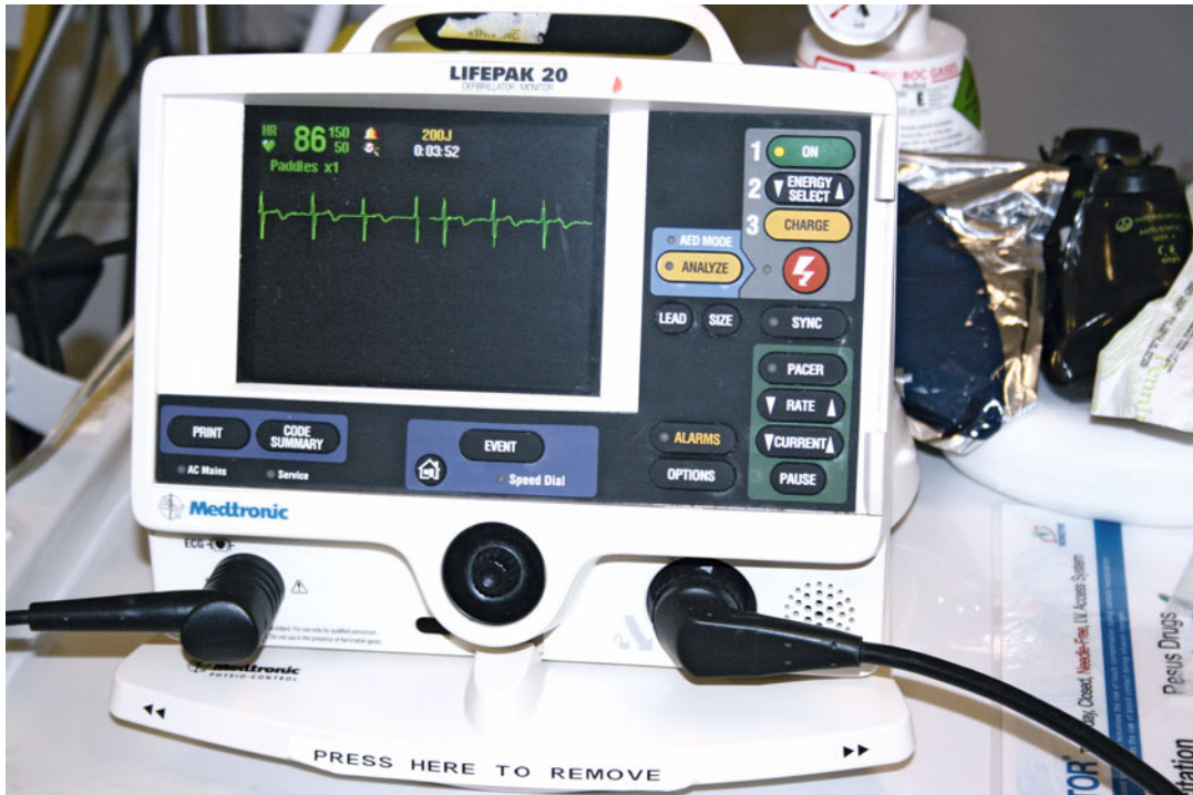
Fig. 13.7 Lifepak 20 (Medtronic Inc.) is both a defibrillator and external pacemaker
