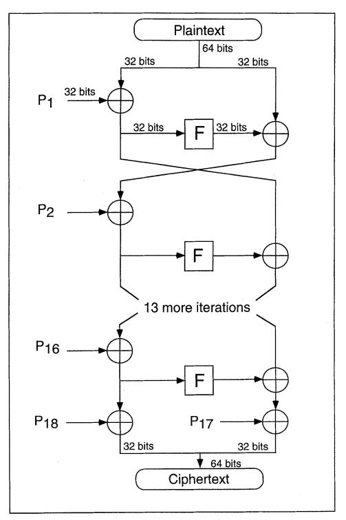
Figure 1: Block Diagram of Blowfish
