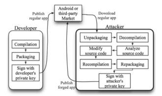
Fig. 2 Android app forgery process which exploits repackaging vulnerability
