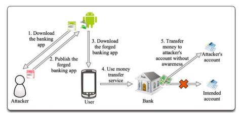
Fig. 8 Attack scenario. An attacker distributes a forged app so that the remittance is made not to the intended recipient, but to the attacker himself
