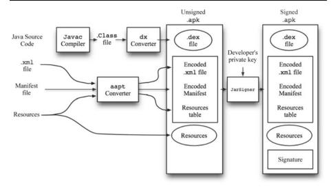
Fig. 1 Android app building process. The series of steps for the building and packaging of files are needed to make up the APK
